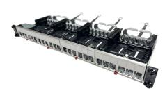
The LCS3 patch panel has been designed and produced to optimize space, with up to 48 ports per unit and to make maintenance and future upgrades easier. It features a quick eject system for loading and unloading a cassette from the front of the rack, and an innovative cable guiding system for tidy and easy cable management. Accepts HDJ (UTP), HDJS (FTP), HDFM, and HDJ AV connectors.
