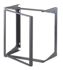
The patented Swing-EZ wall rack arrives ready to square and keyholes mount in minutes. Reinforcement plates stabilize the frame to allow maximum load bearing capacity. Latch pins or bolts secure the door to the frame and remove to swing open smoothly from the left or right.
