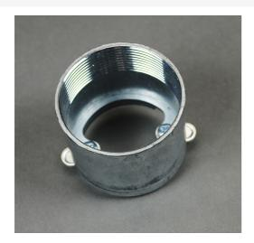
Installed either before or after concrete pour to create activation from duct. NOTE: Drill a 2 1/2in (64mm) hole in concrete and a 2 1/4in (57mm) hole in duct.
