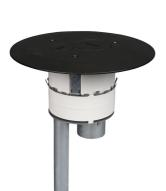
Complete with one-piece finish flange and conduit assembly. Conduit assembly consists of one 3/4inch trade size conduit and one 1 1/2inch trade size conduit. Finish cover flange provided with one 3/4inch trade size screw plug opening and one 1 1/2inch trade size screw plug opening. Covers available in painted black (BK), gray (GY), brass (BS), bronze (BZ), and brushed aluminum (AL). NOTE: Assembled with scrub water gasket. For use on tile, wood or carpet floors.
