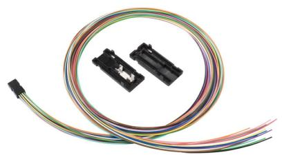
Loose Tube Fiber Breakout Kit, with 12 fibers, each of which are 3 feet (36 inches) in length are used to fan out and build up 250 micron fiber, buffering to 900 microns, when terminating loose tube fiber.
