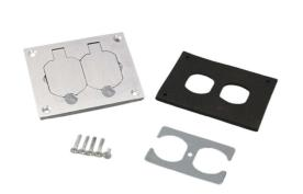
Brushed aluminum duplex cover plate, for OmniBox® and Modulink™ Series floor boxes. Cover plate is 3.290 inch x 4.310 inch (83.6mm x 109.5mm). Flip lids can also be used with 106 type frames for communications. NOTE: Brass covers and flanges are not interchangeable with aluminum or nonmetallic covers and flanges. Nonmetallic covers are interchangeable with aluminum flanges.
