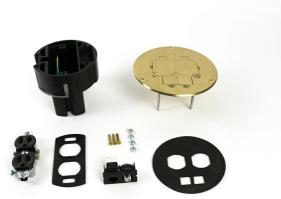
Includes round PVC floor box, one 15A, 125V tamper-resistant duplex receptacle, one coax F connector, one RJ45 Category 5e connector, and brass duplex opening cover plate with two flip lids
