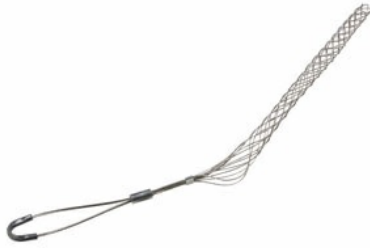
FC0500F: Standard Duty, Closed Mesh, Offset Eye Grips, Cable Diameter 0.50 - 0.61 inches, Bale Length 4-in, Mesh Length 11-in, Break Strength 770 lbs.
