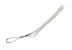
FC1500F: Standard Duty, Closed Mesh, Offset Eye Grips, Cable Diameter 1.50 - 1.74 inches, Bale Length 5-in, Mesh Length 18-in, Break Strength 1680 lbs.
