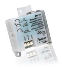
The FM-105 High Frequency Occupancy Sensor is a line voltage sensor that turns lighting on and off based on occupancy, and can hold lights off when sufficient daylight is available. It detects motion via high frequency electromagnetic waves and the Doppler principle. Because it can detect motion through many dense materials other than metal, the FM-105 can be installed behind fixture lenses and hidden from view.
