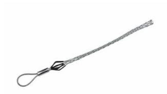
Junior Duty, Flexible Eye. Cable Diameter - 0.500-0.610-inch, Mesh Length - 8-inch, Break Strength - 1,700 lbs.
