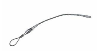
Light Duty, Standard Length, Flexible Eye. Cable Diameter - 1.500-1.990-inch, Mesh Length - 25-inch, Break Strength - 7,500 lbs.
