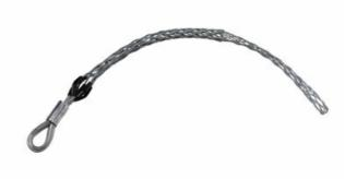
Medium Duty, Short Length, Flexible Eye, T-Type. Cable Diameter - 1.500-1.990-inch, Mesh Length - 24-inch, Eye Diameter - 7/16-inch, Break Strength - 16,400 lbs.
