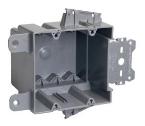
Double Gang, Wood and Steel Stud Bracket Box with Quick/Click, 3/8-inch offset for wood and steel stud mounting. Four Auto/Clamps on each end. For use with 3/8-inch to 5/8-inch wallboard. 50 pack.
