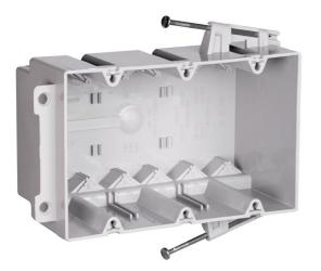
Triple Gang Switch and Outlet Box with captive mounting nails on each end. It has six Auto/Clamps each end with Quick/Click entries. It is easy to install with a rectangular cutout. It is made with a durable, impact-resistant thermoplastic box. It has innovative extras that help cut installation time. Qty 50
