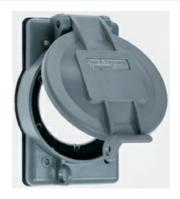
Industrial Grade Weatherproof Lift Cover, 2.32-inch Diameter Opening to Accommodate 20A/30A Turnlok®, For Flanged Inlet/Outlet
