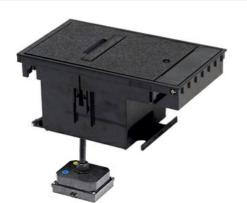
The black Outdoor Ground Box cover assembly is prewired with (1) 30A L6-30R 240V corrosion-resistant duplex receptacles.
