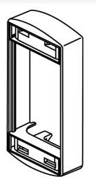
25DTP Kit with 8" (203mm) hole cut cover and mounting adapter. Accepts Wiremold Open System communications modules.
