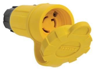
Locking Watertight Connector, 15amp 125volt, NEMA Configuration L5-15, multipoint sealing system provides environmental protection of NEMA 4, 4X, 6, 6P, and IP67 rated.
