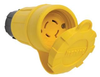
Locking Watertight Connector, 20amp, 3 250volt, NEMA Configuration L15-20, multipoint sealing system provides environmental protection of NEMA 4, 4X, 6, 6P, and IP67 rated.
