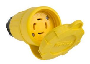
Locking Watertight Connector, 30amp 3 250volt, NEMA Configuration L15-30, multipoint sealing system provides environmental protection of NEMA 4, 4X, 6, 6P, and IP67 rated.
