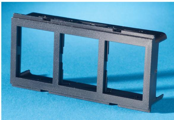
This plate accepts three TracJack modules or blanks. Use with 40700071, 40700072, or 40700073 bezels, to snap mount into 2.70" x 1.375" TIA referenced furniture openings for Steelcase, Haworth, Knoll and others.
