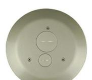
Complete with one 3/4" and one 1 1/2" trade size conduit adapters and closure plugs. Covevrs available in painted black (BK), gray (GY), brass(BS), nickel (NK), bronze (BZ), and forged brushed aluminum (AL). Use with the 4FFSTC15 insert to form a complete poke-thru assembly. NOTE: Assembled with scrub water gasket. For use on tile or carpet floors. 4FFATC Series Poke-Thru Devices require a 4" (102mm) diameter hole.
