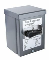
Manual Control Switch 2-Pole 60A 600V in NEMA 3R Enclosure. Slotted opening on enclosures allows for lock-out, tag-out functionality.
