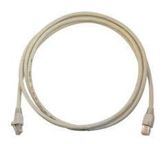
This component rated 500 MHz Cat 6a patch cable fully supports 10 Gigabit Ethernet up to 100 Meters. The snagless boot protects the tab from catching on other cables in a high density patch panel application. These pat
