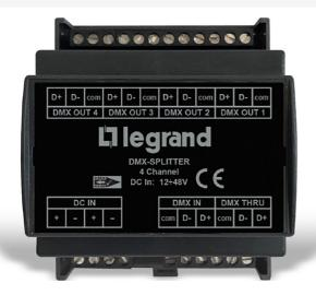
The Wattstopper DMX-SPLITTER is a repeater that divides and regenerates the DMX/RDM input signal into four output channels. It is used with DMX controlled lighting systems when the maximum of 32 devices per bus run is exceeded. In this way, more devices can be added to a DMX network without adding a new DMX-DALI controller. In addition to DMX, the DMX-SPLITTER also distributes RDM messages for devices that use RDM
