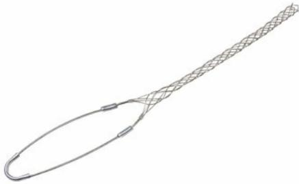
FC062U: Standard Duty, Closed Mesh, Single-Eye Grip, Cable Diameter 0.62 - 0.74 inches, Bale Length 8-in, Mesh Length 11-in, Break Strength 960 lbs.
