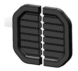
The grommet is designed with 2 half sections for easy installation into any Legrand cabinet with a 4" fan knock-out. Each half contains segmented strips that can be separated to ensure a good seal regardless of the cable bundle size. The strips of each half overlap at the center further ensuring a complete seal.
