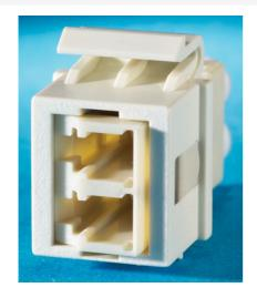
1-LC (2 fibers) fiber Keystone module, multimode, phosphbronze alignment sleeves, 180 degree exit, Fog White
