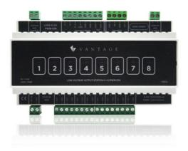
The 0-10 PWM Low-voltage output station (LVOS) is used for the control and automation of LED, CFL, and CCFL lighting loads requiring either 0-10 or PWM for dimming control. The dry contact inputs can be used with motion sensors, light sensors, pressure sensors, IR inputs, magnetic switches, and more. As part of the Vantage lighting solution, it provides control of LED loads as well as inputs from dry contacts for lighting and automation.
