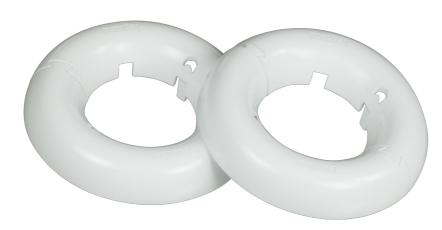
Mighty Mo 20 white Hexguard snaps into the channel rails of the rack and protects copper and fiber cables from cutouts in the channel rails while allowing for easy passage thru the channel. The Hexguard snaps directly into the honeycomb cutouts and can be installed for new, as well as existing cable installs. Kit includes 12 half hexguards.
