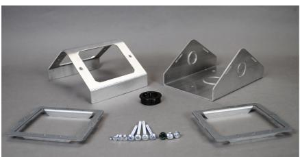
Single-service fitting includes housing, base, two mounting frames, and mounting hardware. For use on 2" (51mm) IPS or PK Preset Systems. For PK activation, use in conjunction with FloorPort Partition Feed and PK Kit. Has 1/2" and 3/4" trade size conduit knockouts on each end. 53.3 cu. in. (906cm3) capacity.
