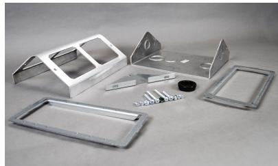
Dual-service fitting includes housing, base, two mounting frames, divider, and mounting hardware. For use on one No. 2 and one No. 4 Duct. Has 1/2" and 3/4" trade size conduit knockouts on each end. 104.3 cu. in. (1709cm3) capacity.
