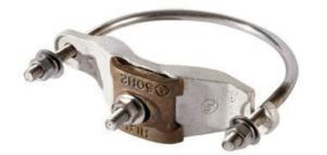
Nominal pipe size range: 3.5" – 4", pipe outside diameter: 3.2" –4.5" Manufactured from electroplated tinned bronze. Conductor range: #6 through 250 MCM PEM stud ensures a flush mounting surface. 5pk.
