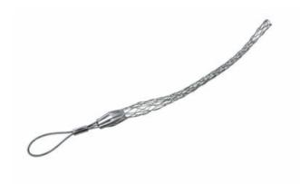
Light Duty, Short Length, Flexible Eye. Cable Diameter - 1.500-1.740-inch, Mesh Length - 16-inch, Break Strength - 7,500 lbs.
