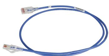
RDC610 Modular Patch Cord, blue, 7', reduced diameter, 28 AWG, cat6a channel four-pair UTP stranded PVC/CM.
