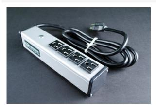
Four outlets, rugged gray aluminum housing, 15A. 6' (1.8m) 14/3 SJT black cord with NEMA5-15 plug. Length 9 1/4" (235mm). Receptacle center-to-center 1 1/4" (32mm). Snap-on, slide-off mounting.
