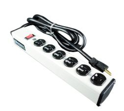
Six 20A, 120V, 60Hz, 2500 watt outlets, lighted switch, putty white aluminum housing, 6' (1.8m) 12/3 SJT black cord with NEMA5-20 plug. Length 13 3/4" (337mm). Receptacle center-to-center 1 1/2" (38mm). Snap-on slide-off mounting.
