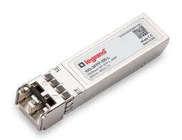
Brocade 10G-SFPP-SR Compatible 10GBase-SR SFP+ Transceiver (MMF, 850nm, 300m, LC Duplex, DDM, I-Temp)
