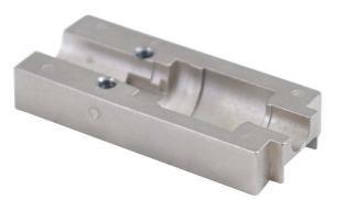
The Visual Fault Locator (VFL) Test Adapter for Simplex SC Infinium Mechanical Fiber Connectors allow the visible indicators in the Infinum mechanical fiber connector to be viewed when using a VFL to ensure cable continuity and determine a pass or fail termination.
