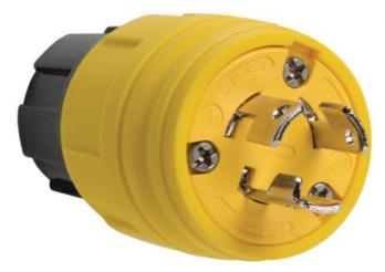
Locking Watertight Plug, 15amp 125volt, NEMA Configuration L5-15, multipoint sealing system provides environmental protection of: NEMA 4, 4X, 6, 6P and IP67 rated.
