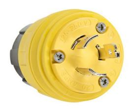
Locking Watertight Plug, 20amp 125/250volt, Non NEMA Configuration, multipoint sealing system provides environmental protection of: NEMA 4, 4X, 6, 6P and IP67 rated.
