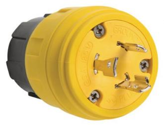
Locking Watertight Plug, 20amp 125volt, NEMA Configuration L5-20, multipoint sealing system provides environmental protection of: NEMA 4, 4X, 6, 6P and IP67 rated.
