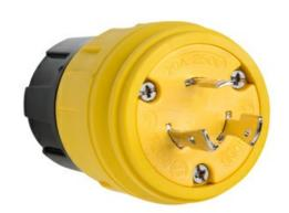
Locking Watertight Plug, 20 amp 250 volt, NEMA Configuration L6-20, multipoint sealing system provides environmental protection of: NEMA 4, 4X, 6, 6P and IP67 rated.
