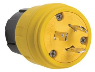
Locking Watertight Plug, 20amp 277volt, NEMA Configuration L7-20, multipoint sealing system provides environmental protection of: NEMA 4, 4X, 6, 6P and IP67 rated.
