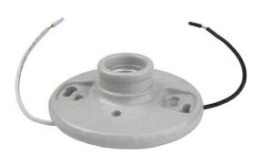
Medium base, porcelain, one piece keyless. 2 terminals with Tamper-Resistant-drive scews, fits 3 1/4-inch and 4-inch boxes, with cage necks, 6-inch Leads.
