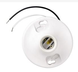
Medium base, phenolic, one-piece keyless, 4 terminals with Tamper-Resistant-drive scews, fits 3 1/4-inch and 4-inch boxes, with cage necks, 6-inch Leads.
