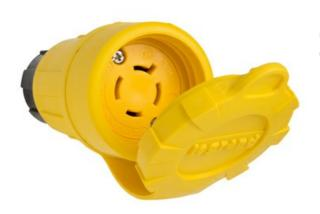
Locking Watertight Connector, 20amp 125/250volt, NEMA Configuration L14-20, multipoint sealing system provides environmental protection of NEMA 4, 4X, 6, 6P, and IP67 rated.
