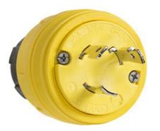
Locking Watertight Plug, 30amp 125volt, NEMA Configuration L5-30, multipoint sealing system provides environmental protection of: NEMA 4, 4X, 6, 6P and IP67 rated.
