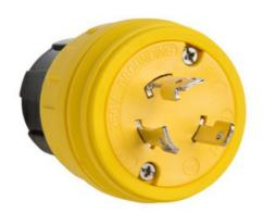
Locking Watertight Plug, 30amp 250volt, NEMA Configuration L6-30, multipoint sealing system provides environmental protection of: NEMA 4, 4X, 6, 6P and IP67 rated.
